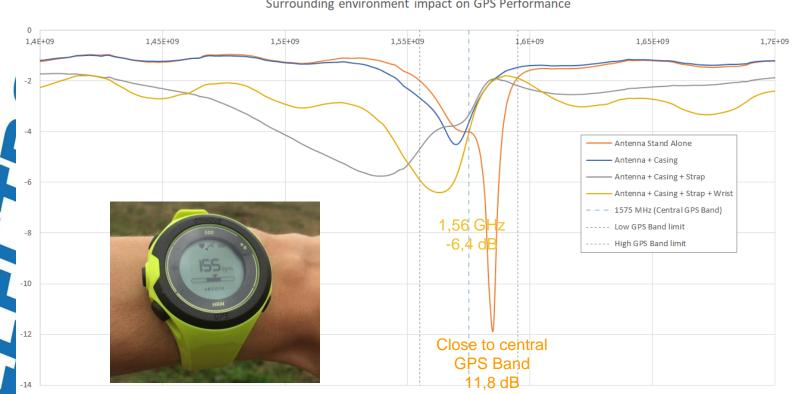
Target of GPS Performance with surrounding environment First Target is to center the frequency 1,585 GHz
